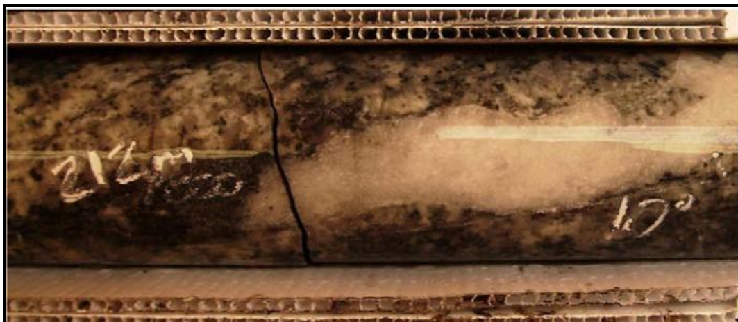
Figure 7.17 White Calcite Vein (Right) Grades into Darker REE-bearing Quartz Vein Tip (Near “212” mark) (LM10-80)
