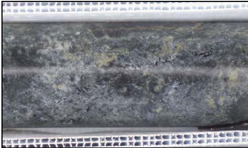
Figure 7.16 Fine Calcite Veining Near the Termination of a REE-bearing Quartz Vein
