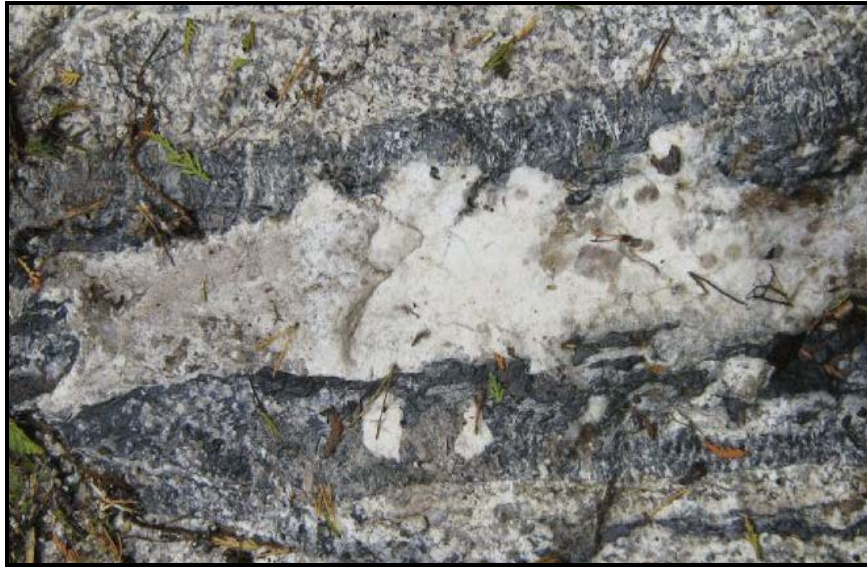
Figure 7.14 Detail of Zoned Vein Showing Sharp, Straight Margins, Lack of Wall Rock Alteration, Ingrowing Marginal Minerals and the Euhedral Central Vein Minerals
